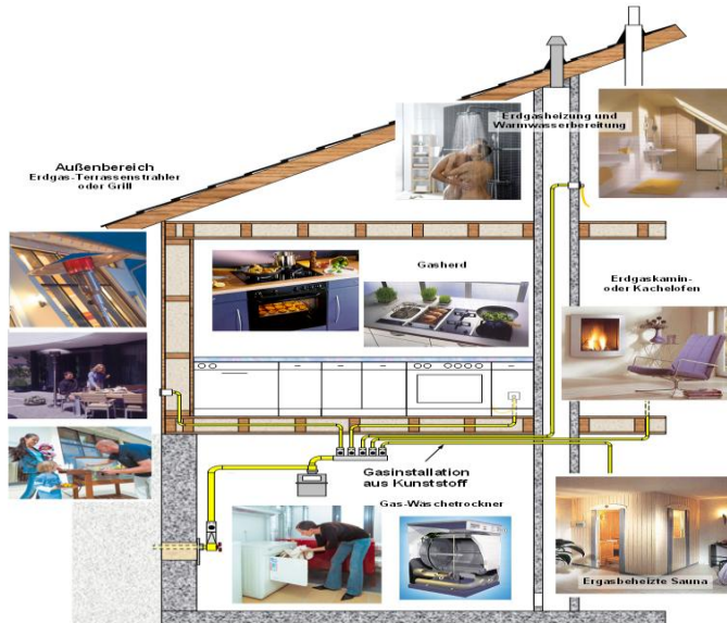
Fig.: New Installation Technologies
